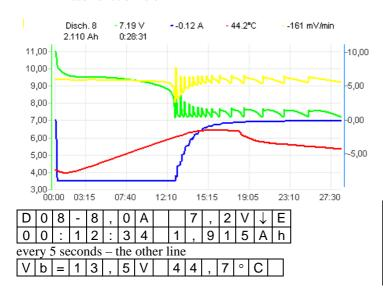
Discharging lasts until battery voltage reaches 0.9V per cell. In *Auto* mode current is decreased by ¼ each time the threshold voltage is reached. Discharging process ends when discharging current is less than 100mA. When *Reverse* mode is set energy from discharging battery is transferred back to the supply accumulator.
