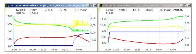
To format a battery means to perform demanded number (1 to 8) of discharging-charging cycles. Discharging is performed in *Auto* mode until 0.9V per cell is reached. Charging is performed in *Simple* mode.
