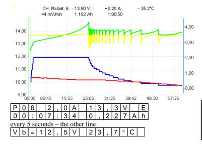
Charging ends when threshold voltage is detected and simultaneously charging current is decreased. When *Fast* function is on charging current is controlled with pulses, which makes it possible to reduce charging time more than two times.
