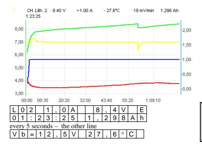
Charging ends when threshold voltage is detected and simultaneously charging current is decreased. When *Fast* function is on charging current is controlled with pulses, which makes it possible to reduce charging time more than two times.
