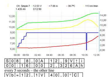
Charging ends when voltage drop  $(-\Delta v)$  or inflexion point is detected. *Inflex* mode allows finishing charging process before unnecessary heating of charged battery starts (inflexion point marker – vertical line on the current graph).
