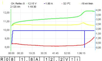
R 08 - charging, 8 cells 1,8A - last measured current 12,2V - last measured voltage
