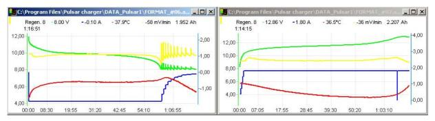
To recondition a battery means to perform demanded number (1 to 8) of discharging-charging cycles. Discharging is performed in two cycles: *Auto* mode until 0.9V per cell is reached and next one with constant current 100mA until 0.6V per cell is reached. Charging is performed in *Reflex* mode.
