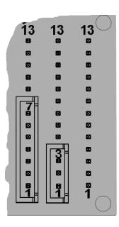
Another example is shown on the left drawing. Here two different XH-sockekts have been soldered to the board. The left one is a 7 pin sokcet for a 6S-accupack and the right one is a 3 pin-socket for a 2S-accupack.
